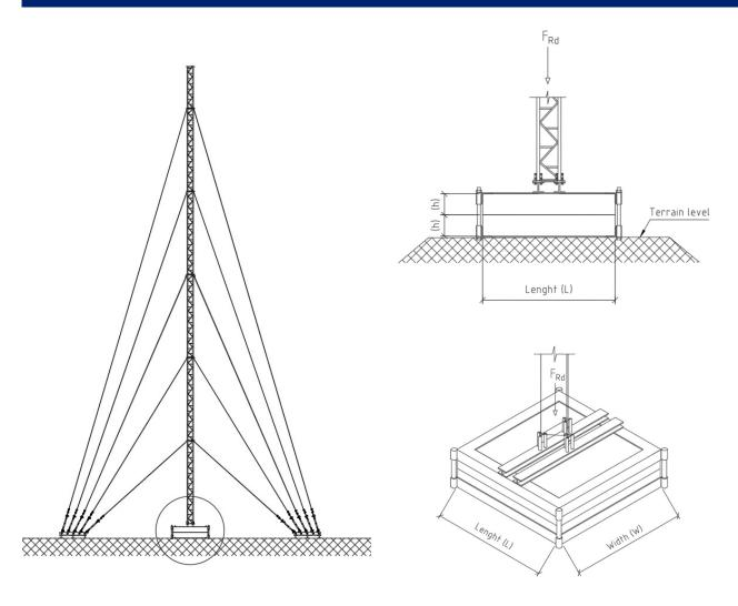
An appropriate foundation solution for a lattice tower mast base is the prefabricated concrete block foundation (B450), which provides, low in time construction, immediate use (no curing/settling).
