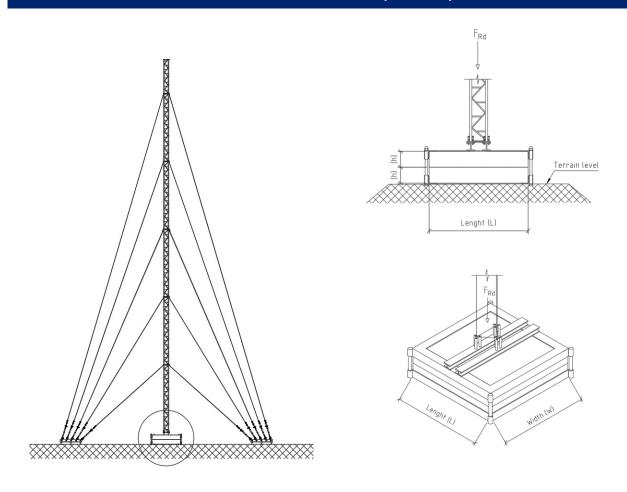
An appropriate foundation solution for a lattice tower mast base is the prefabricated concrete block foundation (B450), which provides, low in time construction, immediate use (no curing/settling).
